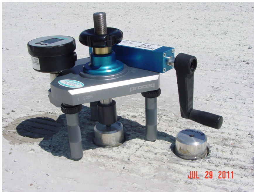
Figure 2.2. Photo - A Proceq-Dyna Z16 Pull-off Tester was used for all pull-off testing.
