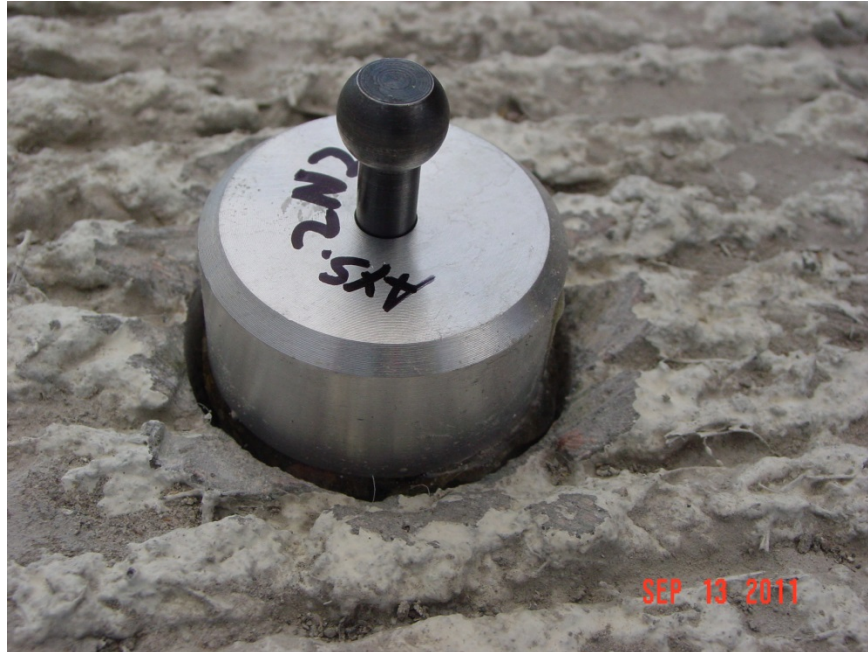
Figure 2.1. Photo - Two-inch diameter, aluminum disk epoxied to the intact drilled core with pull-ball attached. Specimen number was AYS-2N2.
