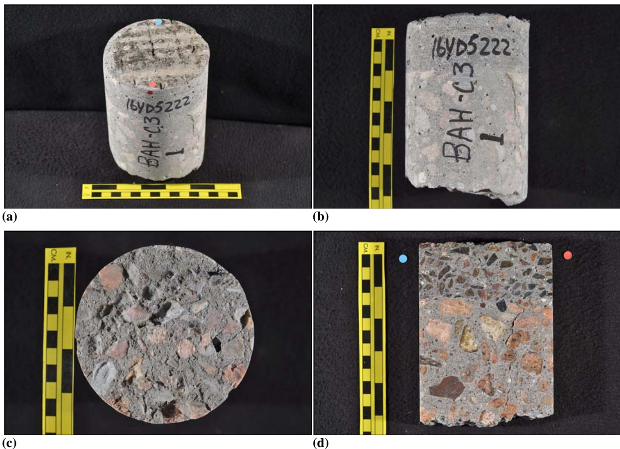
Figure 4.1. Photographs showing example of typical core. (a) Oblique view of the core showing top and side; the red and blue dots indicate the orientation of the saw-cuts used to prepare the sample. (b) The side of the core showing markings used to identify the core. (c) The bottom fracture surface. (d) Polished surface of the core. The yellow scale bar is ~ 150 mm (6 in.) long.
